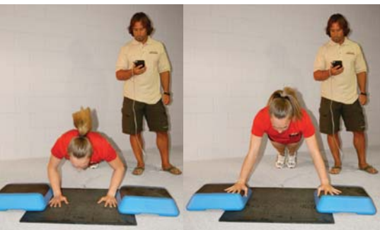
Upper body power can also be accurately measured with the JJR with a plyometric push-up. Here the athlete puts her hands on two low platforms between the force plate, then drops into a push-up and then springs back to the platform.
