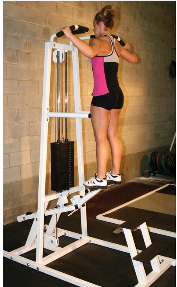
On the BFS Assisted Chin/Dip machine, a footplate is connected through a pulley mechanism to a selectorized weight stack. The more weight you add to the weight stack, the more upward force is applied to the footplate and the less strength is required to perform the exercise.
