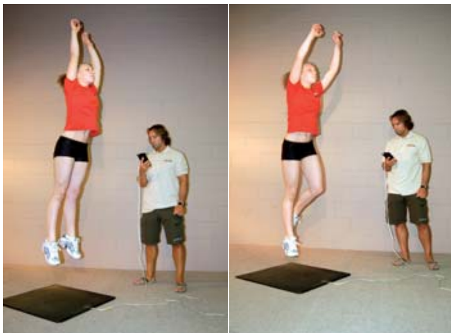
The BFS Just Jump and Run is a force plate that offers a fast and accurate way to test many types of jumps, including single leg jumps.
