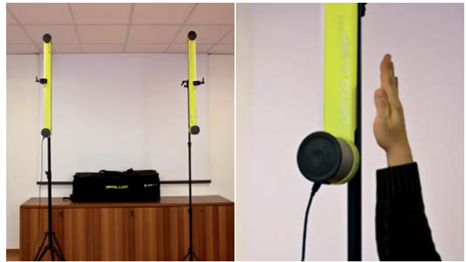
The OptoJump can duplicate the traditional vertical jump testing, and also provides a “Drift Protocol” to determine an athlete’s dynamic stability.
