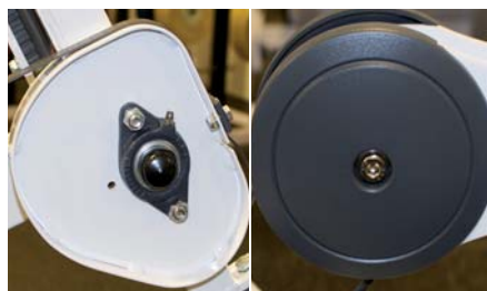
The design of the pulleys on machines affects the resistance curve of an exercise.
