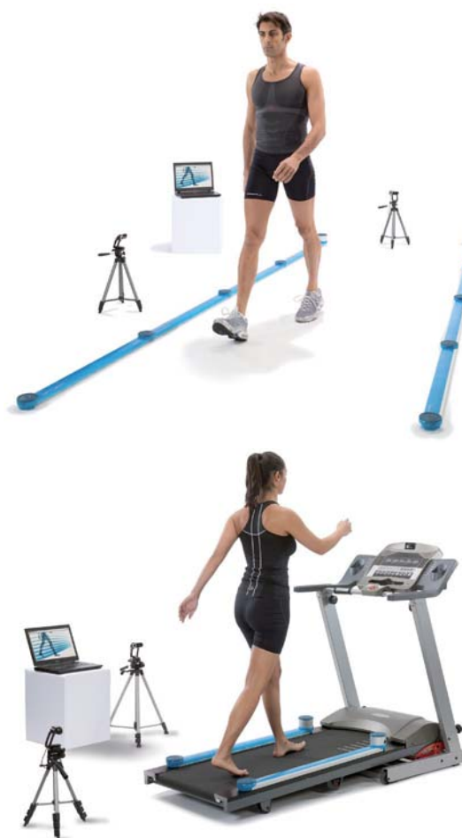
The OptoJump can measure balance control whether the individual is walking, walking on a treadmill or performing complex jumping drills.
